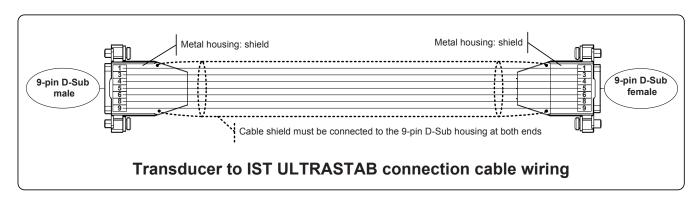
To prevent any malfunction that may occur due to the cable/wire voltage drop (i.e., its length and the wire resistance inside the cable) between the IST ULTRASTAB rack and the transducer, a cable with at least 7 wires, each having a cross section AWG 22, AWG 23 or  $\geq$  0.25 mm², must be used.
