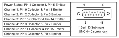
All signals on the status/interlock connector are optically isolated, photocouplers type, floating Collector and Emitter.
